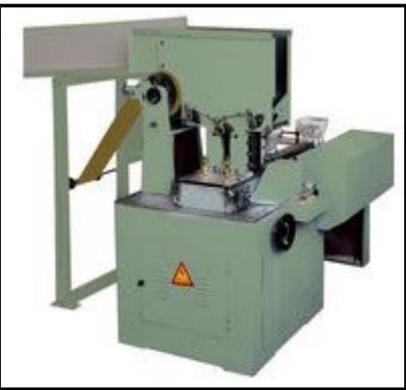
Sharpening and Chamfering Machine
